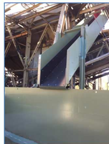
Photo 2 – Completed repairs to transfer house noise curtain, sound barriers around rotary breaker and the new noise attenuated reject chute of the site's rotary breaker.
