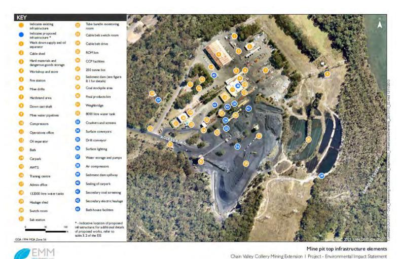
Figure 1 : General Arrangement of the Chain Valley Colliery surface facilities site
