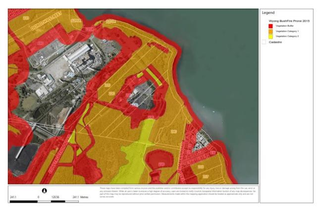
Figure 19 - Bushfire Prone Land Map for Ventilation Shaft Area (Source: Central Coast Council, 2022)
