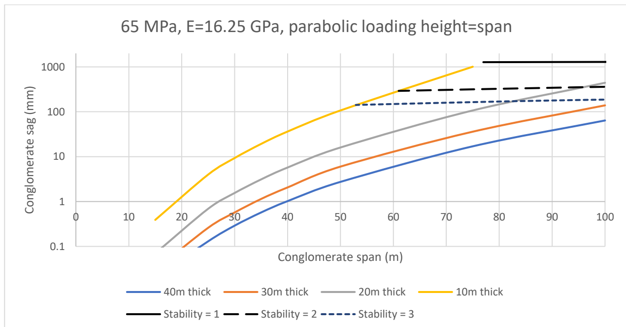
Figure 20 Sensitivity study of the deflection and stability of conglomerates relative to span and conglomerate thickness – 16.5m spans
