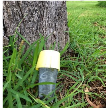
Figure 3: Example of subsidence monitoring point with safety cap
