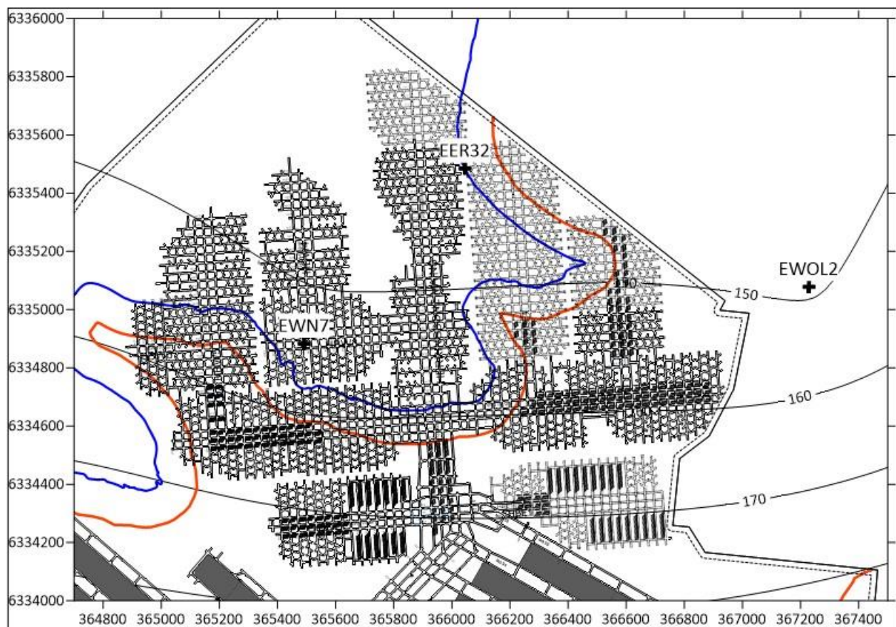
Figure 1 Proposed mine plan showing location of proposed stripping or lifting (black hatched areas), depth of mining, lake edge, seagrass protection barrier, and boreholes
