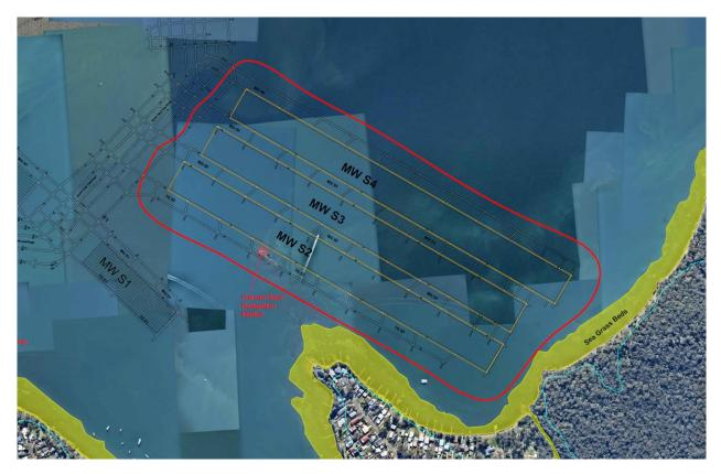
Figure 2 - Predicted Subsidence after extraction of S2, S3 and S4 panels (Hill, 2019)
