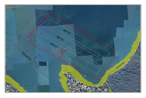
Figure 1- NMD S2 to S4 Extraction Impact area due to Fassifern Miniwall Mining
