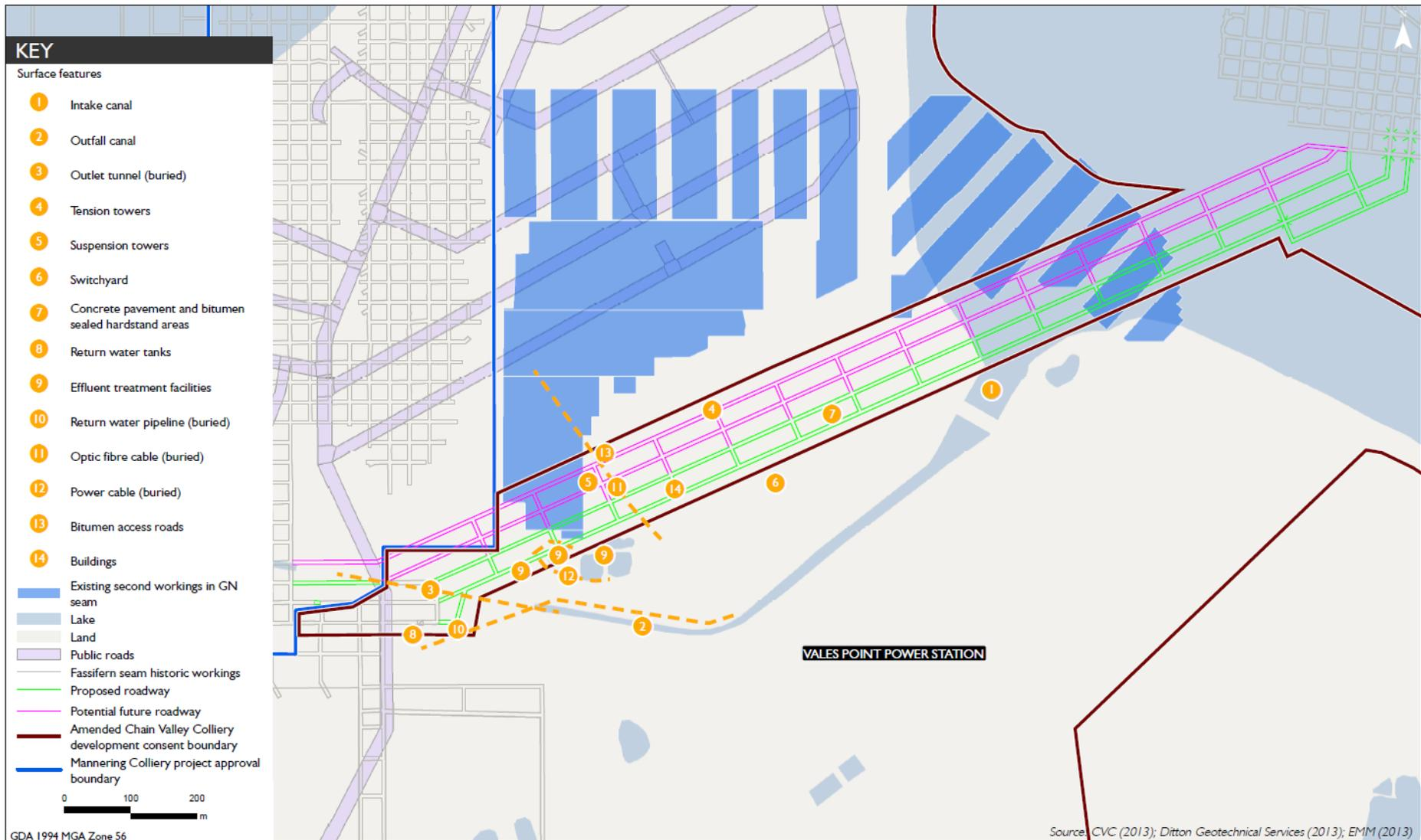
**Figure 3: Location of the underground linkage and surface infrastructure**
